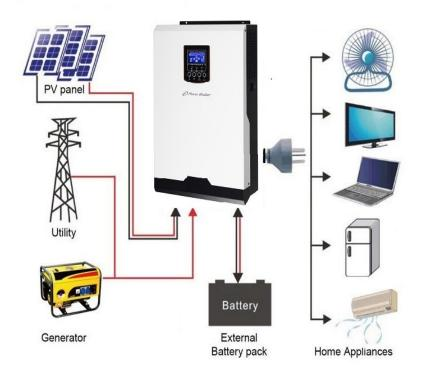
The following illustration shows basic application for this multi-function inverter/charger. It can be used with utility or generator as input source. Configurable external battery setup for backup function (optional available).
